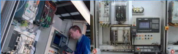
Our Siemens 840C test fixture can test both analogue and Digital drive systems.
