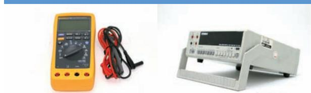
Multimeters, oscilloscopes, function generators, meggers, tachometers and much, much more.
